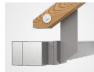
Rafter bracket installation
